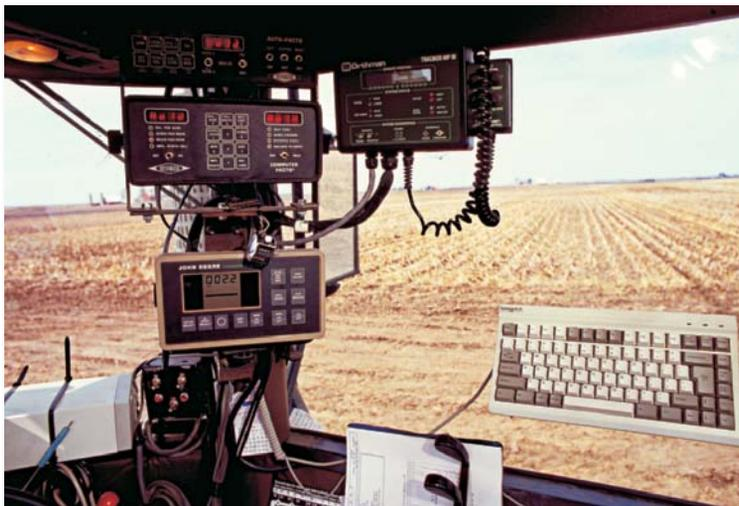
**Soil Mapping** The GPS system, combined with a computer on board the tractor, allows the farmer to map each field to determine how much fertilizer and pesticide each area will need before planting. *How will this knowledge save the farmer time and money?*
